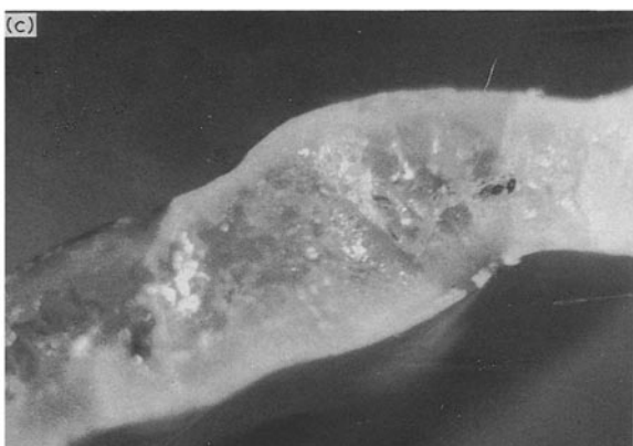
Figure 1 Optical microscope pictures of sections of PLA 50 parallel-sided plates: (a) initial aspect; (b) after 35 days in vitro in non-buffered water; and (c) after one month osseous implantation in sheep.
